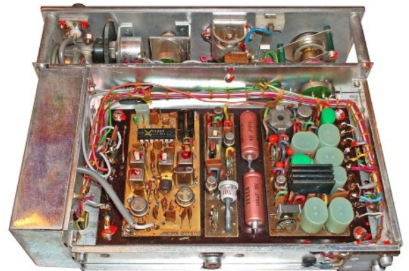
Top and bottom chassis view of Bodrog B spy bug receiver. The unit behind the metal screen at the side is the down converter.
