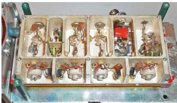
Down converter with cover removed.
